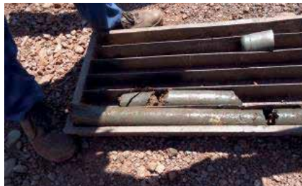
Improved core recovery is visible in the black mudstone after introducing AMC COREWELL™.
