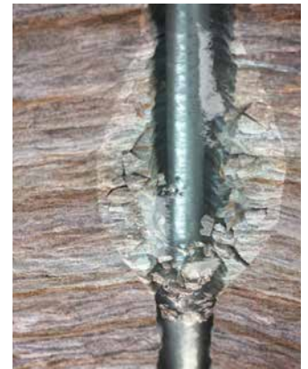
Reactive clay rich formations are susceptible to washouts, the hole wall can become unstable and collapse.
