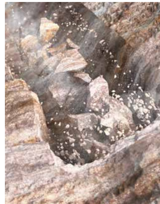
Drilling in unconsolidated and reactive formations can result in poor core recovery.
