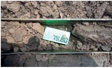
Poor core recovery is visible in the black mudstone.
