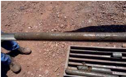
Improved core recovery is visible in the black mudstone after introducing AMC COREWELL™.
