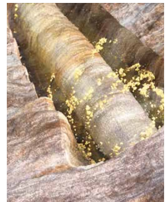
A polymetric network forms a web-like protective barrier, holding the core together as it travels to the surface.
