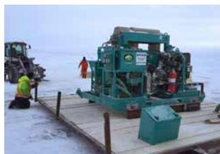
Left: All components of the AMC HP SRU™ weigh under 700kg and can be easily dismantled for transport. Right: AMC HP SRU™ was quickly configured on site.
