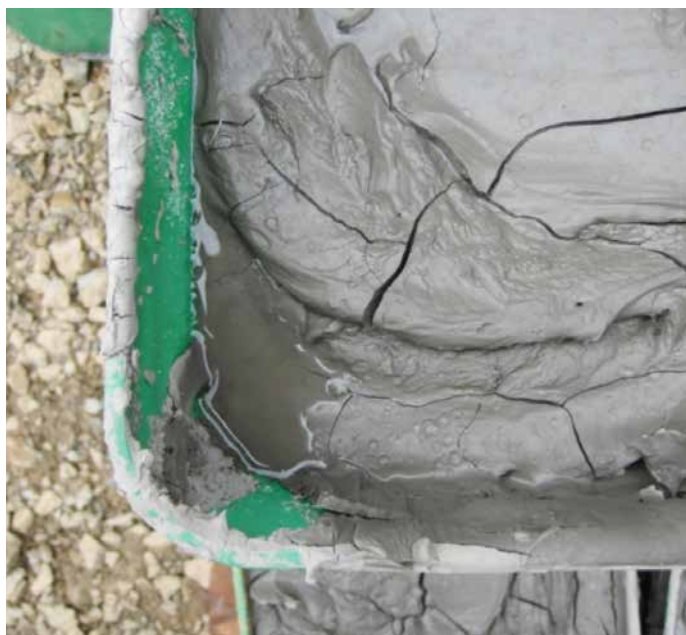
Dry and stiff cuttings after using the AMC Surface SRU™.
