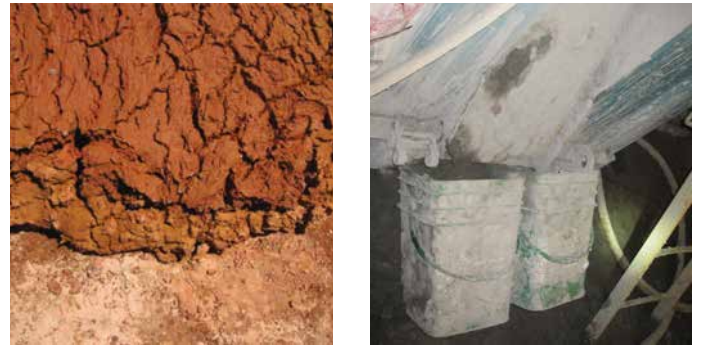
Cuttings have a semi-dry consistency once processed by the centrifuge.
