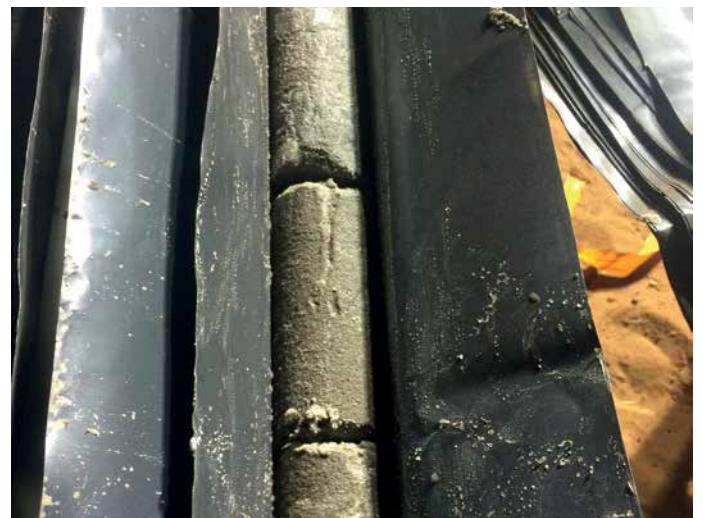
Core recovery after AMC RESI DRILL™.
