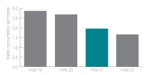
Note: Hole number 22 presented a lithology consisting of mainly compacted ground, therefore water consumption was naturally low, while hole 21 presented a semicompact ground with highly fractured zones.
