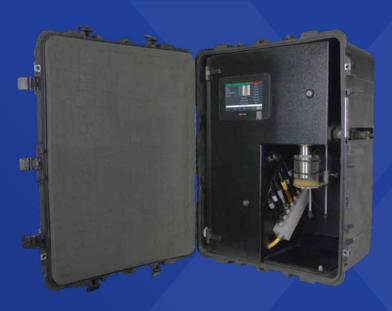
When a drilling fluids specialist cannot be on site full-time, an automated system can be beneficial to measure and monitor drilling fluid properties. The newly launched IMDEX MUD AID™ is a remotely monitored, Automated In-field Diagnosis unit, designed to manage and automate drilling fluid processes.
